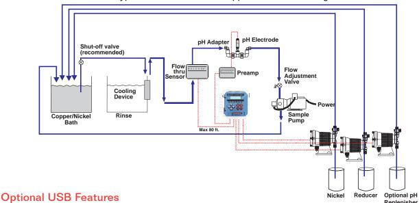
Integrated datalogging collects analytical measurements at 10 minute intervals and captures all relay activations.
