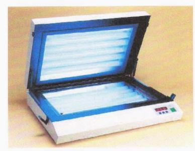
The AZ220 double sided vacuum UV should be considered an essential part of any system for manufacturing double sided PCBs. The ability to expose both sides of the board at once eliminates the immense problem of artwork registration for two separate exposures on a single sided unit.
