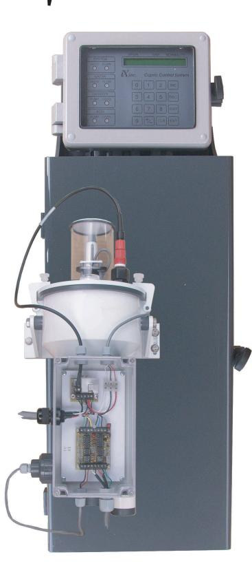
The CP-1 cupric control system provides a complete chemical control package for the control of cupric chloride etchant. Copper, Acid normality, and oxidation potential are independently measured and controlled using a time proven analytical procedure. The system monitors both internal and external systems for faults and alerts the operator with an audible alarm.
